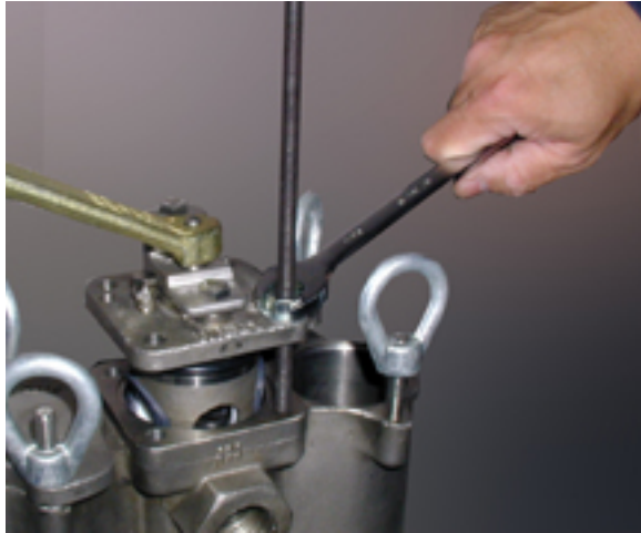
Photo 9: The cartridge insertion / extraction tool is used to finish installing the cartridge into the strainer body.
