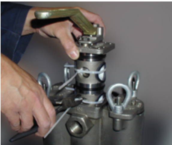
Photo 7: When the ball, seats and seals enter the strainer body the restrainer ties are cut.
