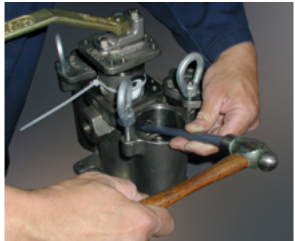
Photo 8: The seal insertion tool is used to push the seals past the body ports on both sides of the strainer as the cartridge is reinstalled.
