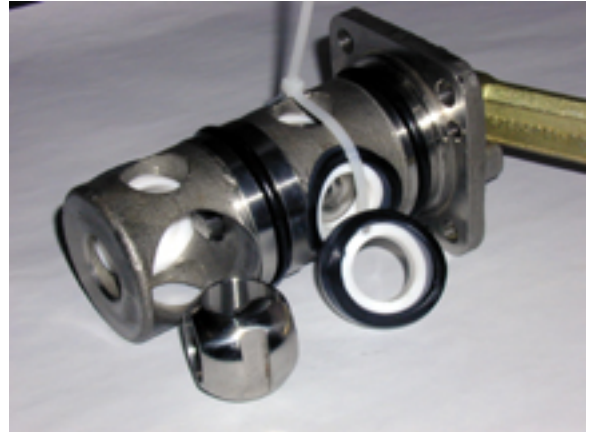
Photo 6: Once the cartridge is removed the balls, seats and seals can be inspected and replaced as necessary. The restraining ties are put back in place prior the cartridge being reinstalled back into the strainer body.
