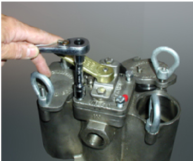
Photo 11: Tightening down the cartridge hex head screws completes the installation of the cartridge back into the strainer body.
