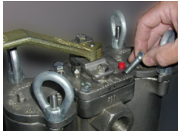
Photo 2: Unscrewing the hex head screws allows the cartridge to be removed. The red cap protects the threaded connection used by the insertion / extraction tool.
